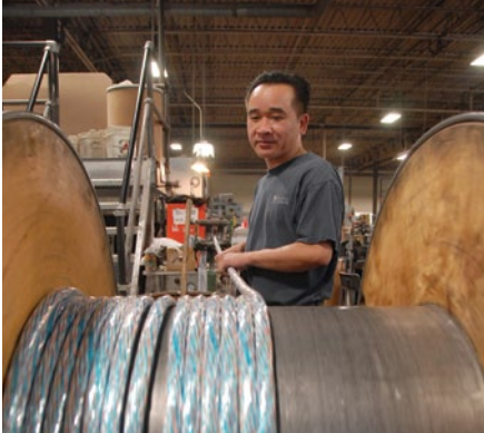
STAGE 4: The jacket extrusion process culminates with ink-jet printing.
